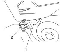
14. Remove the dipstick (2) and add two quarts (1.9 l) of the recommended oil. Reinstall the dipstick.
